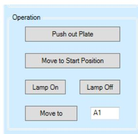
**Push out Plate:** Moves the plate to a position from which it can be easily removed from the Microplate Reader Accessory.
