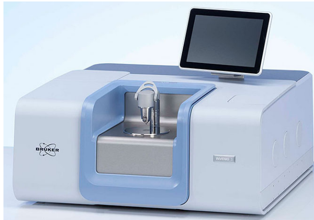
Figure 2.3: INVENIO S with integrated ATR unit
