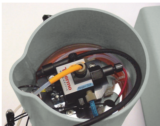
Figure 68. Dionex CR-TC installed in Dionex EGC holder
