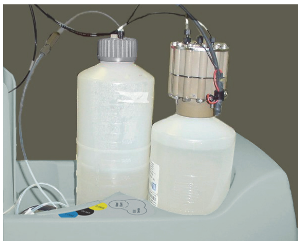
Figure 76. Dionex EGC in service area
