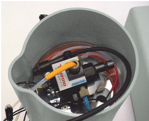
Figure 80. Dionex CR-TC installed in Dionex EGC holder
