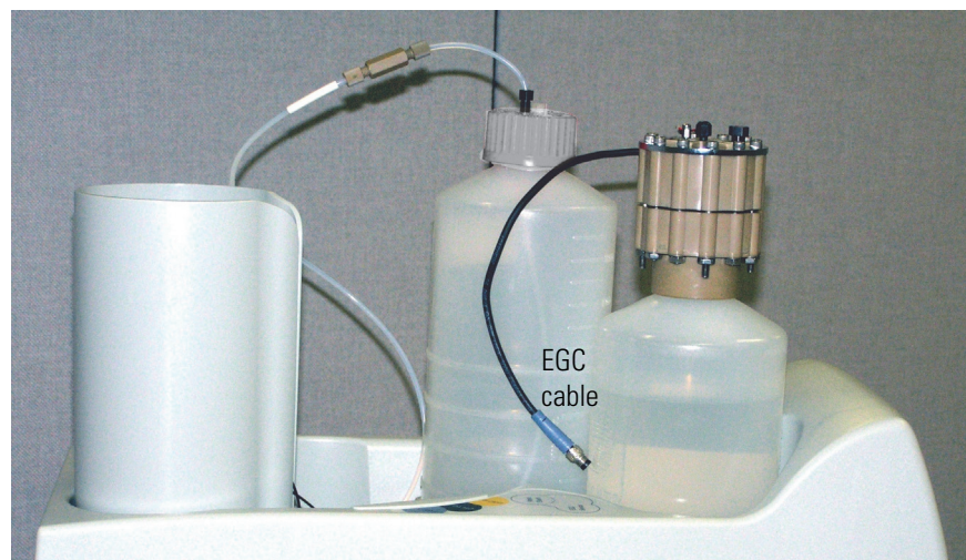
Figure 61. Dionex EGC in the service area
