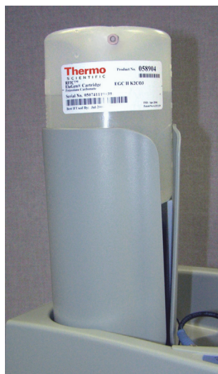
Figure 62. Dionex EGC installed in the holder
