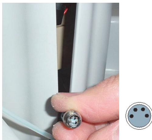
Figure 54. Connecting the Dionex EGC electrical cable
