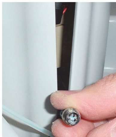
Figure 63. Connecting the Dionex EGC electrical cable
