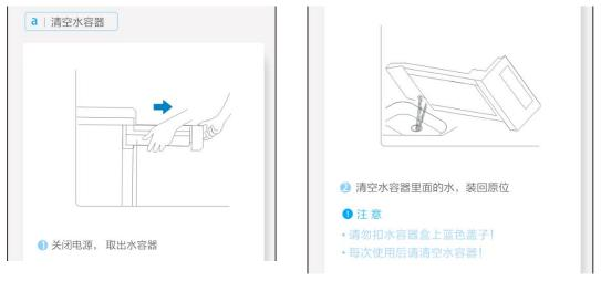
Cut off the power then empty the water container (In the upper left of the Dryer)
